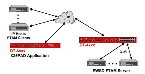
In the diagram above, the FTAM clients on the TCP/IP hosts communicate with the **X25PAD** application in the native RFC1006 FTAM protocol. The **X25PAD** mediates with the ISO based X.25 implementation of the FTAM protocol. The physical X.25 links are connected to a **DT-4xxx** serial port remote from either the **DT-6xxx** or the FTAM client hosts.
