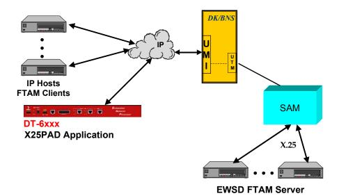
In the diagram above, the only change made was a UMI as the mediation point between the TCP/IP network infrastructure and the BNS/DK network infrastructure. Any variant of SAM may be used for the serial connection. Options include the SAM 64/504, a **DT-4000**, and the **DT-SAM**. The SAM and DK/BNS node need not be collocated with each other or with the DT-6xxx on which the X25PAD application resides.
