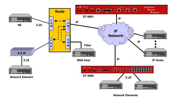
In the above configuration, there is one circuit carrying X.25 LAPB frames from the DT-6061 to a DT-4000 connected Network Element (NE) or a SAM connected NE. The X.25 Network Element may be anywhere on the available networks (both BNS and IP) as the above diagram depicts. IP Hosts access the virtual circuits on these Network Elements via a TCP port number. BNS Hosts
