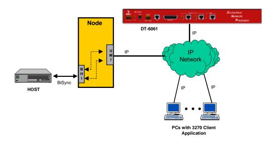
In the above diagram a 3270 client would call the BiSync host using the IP address of the DT-6061 plus the TCP port assigned to the TN-3270 server **instance**<sup>1</sup> which is assigned to a line on the Bisync host.
