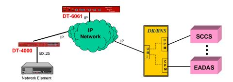
In the example above, the BX.25 network element has a synchronous HDLC connection with a DT-4000 port. The DT-4000 port is configured as *standalone originate* to the TCP port on the DT-6061 terminating the X.25 line. The SLM function is in the aggregate of all the LCNs present on the BX.25 link. Individual LCNs are processed individually, but the interface with the NDC/OS is the internal SLM protocol on a single connection.
