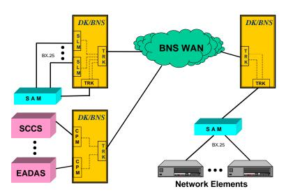
The diagram above represents a typical deployment for some RBOCs. Others will directly connect the Network Elements on the SLMs via 202T modem sets or equivalent. In the diagram, the SAM at the Network Element site acquires the BX.25 and transports it transparently to the SAM co-resident with the SLM modules. The co-resident SAM is used merely to provide centralized connectivity with the SLMs. Such an arrangement has also been done with Transparent Synchronous Modules (TSM).
