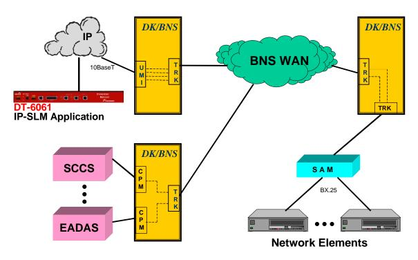
Note: Each DT-6061 using the IP-SLM application will support 30 Network Elements. Each UMI will support 250 Network Elements since two circuits are used per NE.
