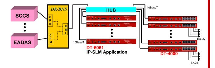
In the diagram above, there is support for 450 individual BX.25 lines from the Operations System via the UMI. There are also 24 sessions available for access to the network for OA&M and other functions. Please note that the Network Elements are attached via a 202T or similar modem device.
