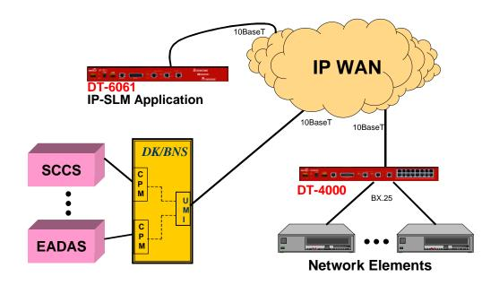
In the diagram above, the IP network may be a simple hub if a private network is desired. The DT-4000 ports are used to connect the BX.25 network elements. These may be co-located with the DT-6061, or may be co-located with the Network Element, as is required. The UMI provides the connectivity to the Operations Systems.
