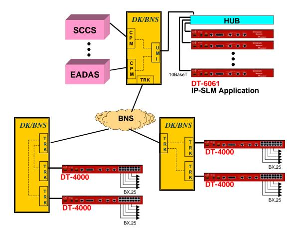
In the diagram above, the DT-4000's are operating in their SAM16 emulation. The DT-4000 can support this emulation and have standalone functions simultaneously.
