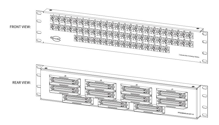
CBM of America's PPSAM64RJ45-50T-19 accepts pre-existing 50-pin cables with CHAMP-style connectors (50-pin "Telco" connectors) from Datakit SAM/64s. It provides 64 RS-232 ports on RJ-45 connectors, pinned according to the Cisco and MRV convention. The PPSAM64RJ45-50T-19 occupies two RU in a 19-inch rack. All 50-pin connectors can be secured with included hook-and-loop straps or with included bail locks (neither shown in rear view for clarity).
